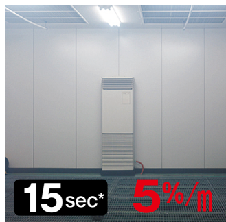
Transition of smoke density (attenuation rate %/m) of smoke emission specimen (results of experiment conducted by Fenwal Controls)
